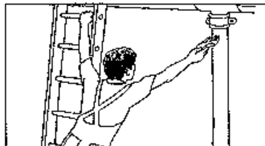
Figure 1. Don't do this— MOVE the ladder!
